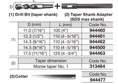
SDS-plus Shank Bit Adapter (SDS max shank)
